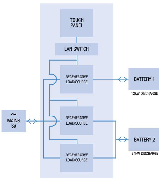
Figure 1 - Independent testing of 2 different types of batteries
